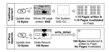
Figure 1: Write-amplification: traditional vs IPA.
