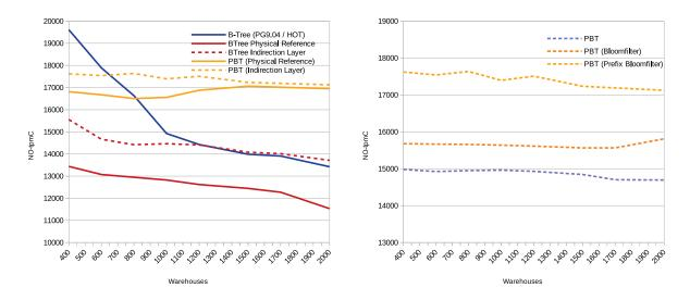
(a) Indirection Layer vs. Physical Tuple Reference (b) Influence of Filter Techniques on Throughput
