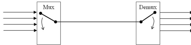
Figure 9.17 Example of a multiplexor and demultiplexor application
