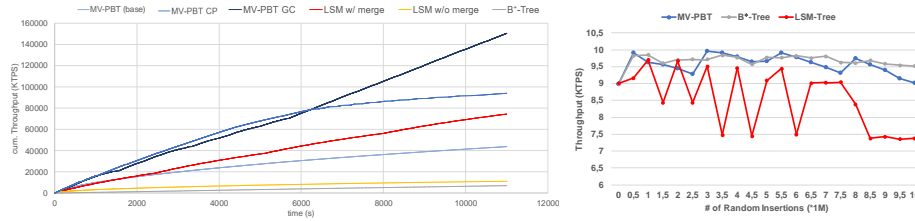
(a) Accumulated executed transactions (*1k) in YCSB Workload A with 1kB value size (b) Intermediate State Read-Only Throughput
